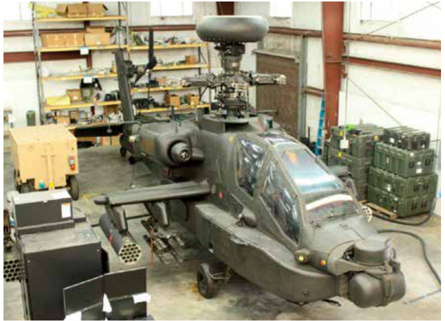
The L-7AY Multiplex, Avionics, Visionics, Weapons, Electrical Systems Trainer (MAVWEST) during acceptance testing at Joint Base Langley-Eustis, VA.
