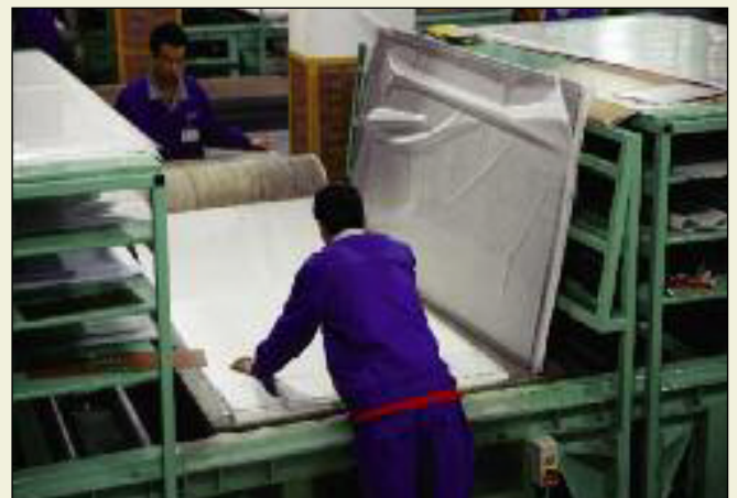
Deeper embossing during the hot press process allows for crisper, more realistic-looking visuals, according to Metroflor.
