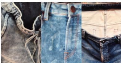
Eco-Friendly: Waterless finishing using lasering by Jeanologia.
