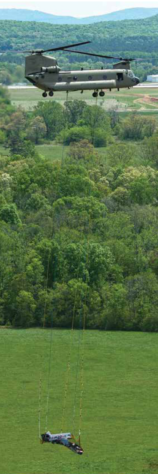
A CH-47F recovering a damaged MQ-1C Gray Eagle with the Modernized Unit Maintenance Aerial Recovery Kit (M-UMARK)
