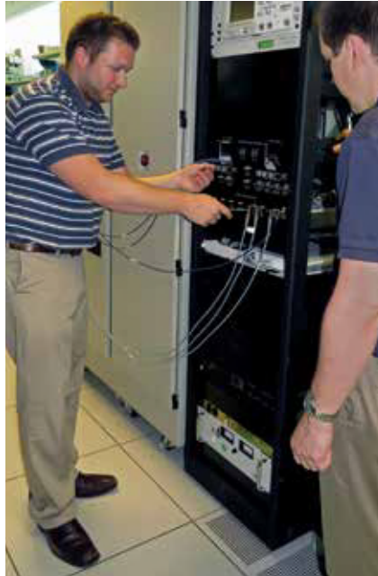
ARAT-PO engineers set up the dual testing Common Automated Test Station (CATS) rack attached to an RF simulator.
