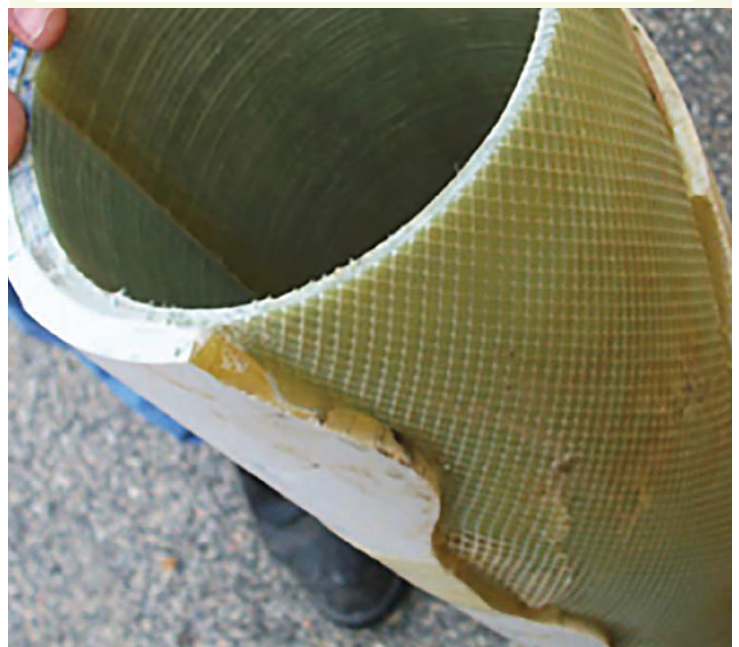
Field testing shows the strength of IRSI repairs; the original pipe cracked, but the IRSI repair stayed intact.
