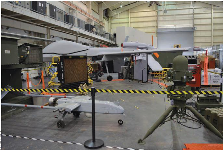
Shown here are unmanned aircraft undergoing hardware-in-the-loop testing at the UAS Joint Systems Integrated Laboratory (JSIL). Interoperability profiling advancements have been made as a direct result of this extremely important partnership between PM UAS and the JSIL, both located on Redstone Arsenal, AL.
