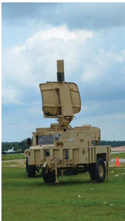
Air Traffic Navigation, Integration, and Co-ordination System (ATNAVICS) set up and ready for flyability check during a field training exercise in July, 2013.
