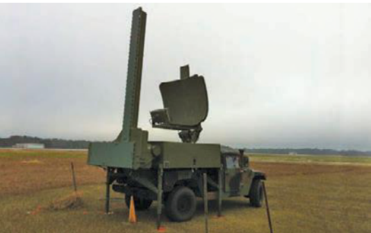
Air Traffic Navigation, Integration, Coordination System (ATNAVICS) is a mobile radar that provides primary and secondary surveillance at tactical airfields.
