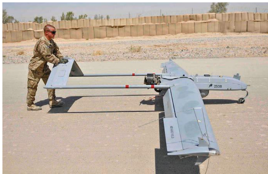
SPC Justin Waltho with Headquarters and Headquarters Troop, Combined Task Force Dragoon, pushes an RQ7B Shadow Tactical Unmanned Aircraft System to a mechanical station to conduct post-flight checks Sept. 12, 2013, at Forward Operating Base Pasab, Afghanistan.
