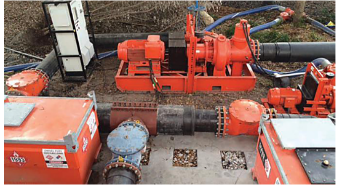
Top: The fuel cubes, lower right and left, were used as part of the back-up redundancy of the system for the diesel driven pumps. Bottom: Space was limited under the expressway and along the river.
