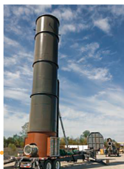
ZEECO Trailer Mounted Enclosed Rental Flare
