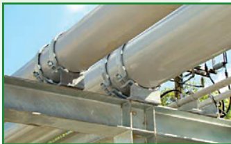
Pipe Shoes are fitted with I-Clip Liners to create minimum bearing surface on pipe allowing air-to-flow, drying moisture and condensation.
